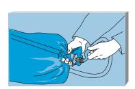
1 Remove the sterilized items only after the sterilization cycle and 2-hour purge cycle have been completed and the display indicates "UNLOAD STERILIZER". The sterilizer will continue to aerate items that are not removed immediately. A count-up timer on the display will indicate additional aeration since the final 2-hour purge cycle ended.
